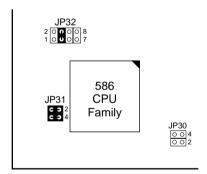
Figure 2–2–2. Single Voltage 3.52V CPU (Default)
