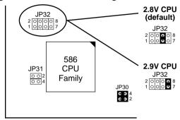
Figure 2-2-3. Dual Voltage CPU
