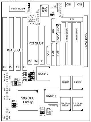
Figure 1–3. Regular Mainboard Default Setting
