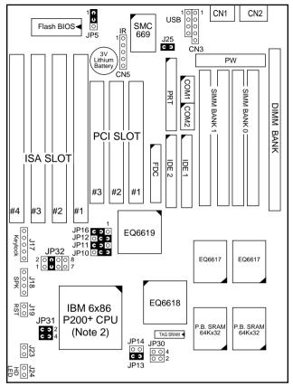
Figure 1–2. IBM CPU Attached Edition Mainboard Default Setting
