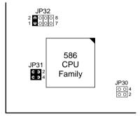
Figure 2–2–1. Single Voltage 3.3V CPU
