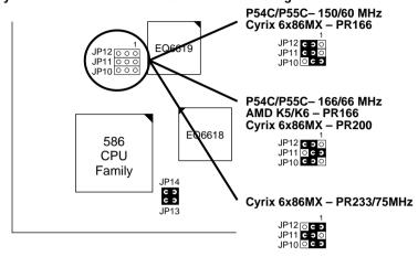
Figure 2–1–3. CPU Jumper Settings
