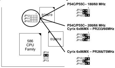
Figure 2–1–4. CPU Jumper Settings
