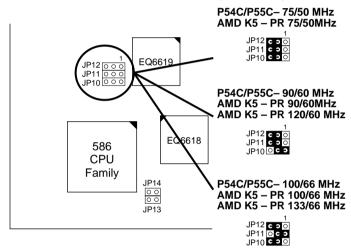
Figure 2–1–1. CPU Jumper Settings
