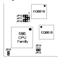
Figure 2-1-3. CPU Jumper Settings
