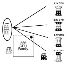
Figure 2-2-3 Dual Voltage CPU
