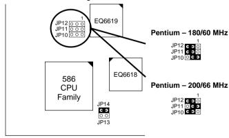
Figure 2–1–4. CPU Jumper Settings
