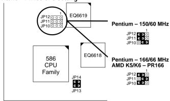
Figure 2–1–3. CPU Jumper Settings
