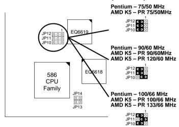
Figure 2–1–1. CPU Jumper Settings
