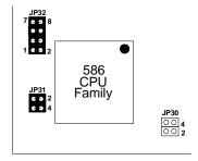
Figure 2-2-2. Single Voltage 3.5V CPU (Default)
