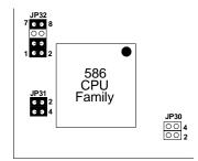
Figure 2-2-1. Single Voltage 3.3V CPU
