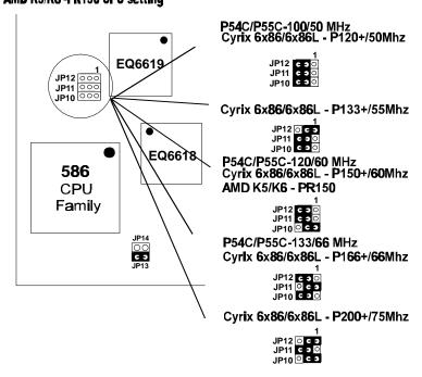
Figure 2-1-2. CPU Jumper Settings
