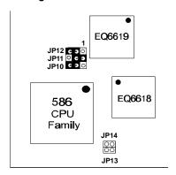
Figure 2-1-2. CPU Jumper Settings
