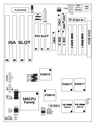
Figure 1-2. Mainboard Default Setting
