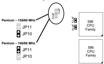
Figure 2–1–3. CPU Jumper Settings
