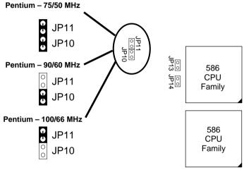
Figure 2–1–1. CPU Jumper Settings
