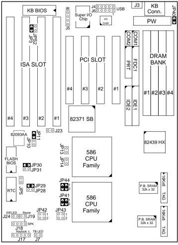
Figure 1–2. Mainboard Default Setting
