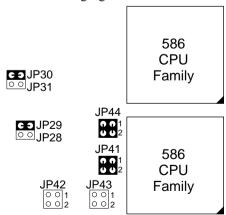
Figure 2–2–1. Single Voltage 3.3V CPU
