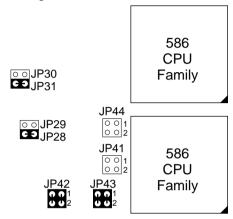
Figure 2–2–2. Intel P55CX (VIO = 3.3V, VCore = 2.8V)
