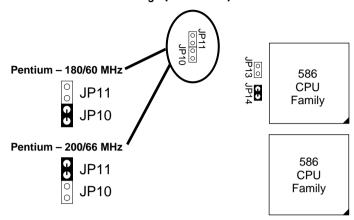
Figure 2–1–4. CPU Jumper Settings
