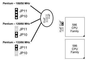
Figure 2–1–2. CPU Jumper Settings
