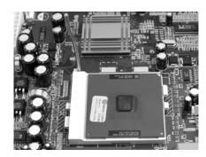
Step 3 Close the socket by closing the actuation lever.
