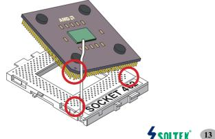
3. Make sure that the CPU position in the socket tightly, and then put the lever down to complete the CPU installation.
