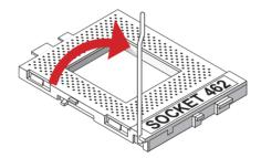
2. Take note of the red circle as below picture. While inserting the CPU into the socket, you can find out there is a definite pin orientation for CPU and socket.
