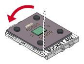
Make sure that the CPU is placed into the socket tightly. Then lower down the level to complete the CPU installation.
