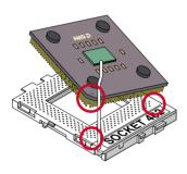
Take notice of the red circles as shown below. While inserting the CPU into the socket, you can find out there is a definite pin orientation for CPU and socket.
