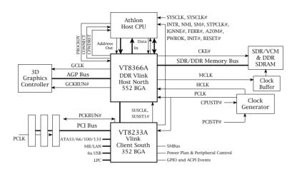
Diagram of Apollo Pro266A System Block Using the VT8233A V-Link South Bridge
