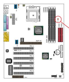
NOTICE: When LED "ZD1" is on, meaning that 2.5V is operating and flowing into DIMM slots, please do not add or remove memory modules.
