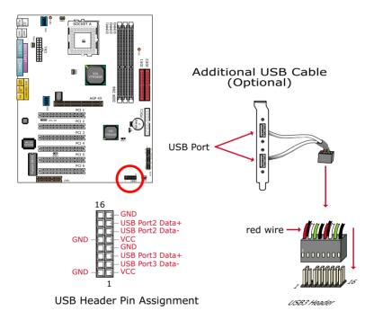
When plugging the USB cable into Header USB3, user must make sure the red wire is connected to Pin 1.
