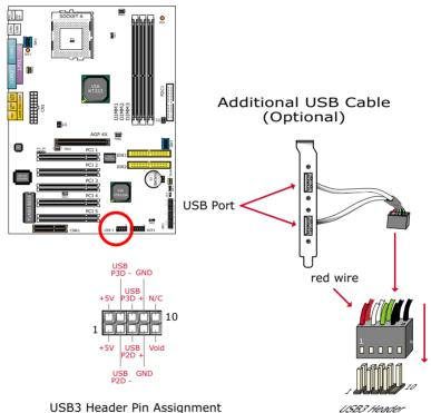
• When plugging the USB cable into Header USB3, user must make sure the red wire is connected to Pin 1.
