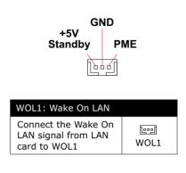
This connector connects to a LAN card with a Wake On LAN output. The connector powers up the system when it receives a wake-up packet or signal through the LAN card.
