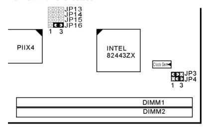
Figure 2-3. CPU Type Configuration
