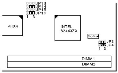
Figure 2-1. CPU Type Configuration
