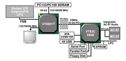
Diagram of VT8601T APOLLO PLE133T System Block with VT82C686B PCI-to-ISA South Bridge
