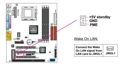
This connector connects to a LAN card with a Wake On LAN output. The connector powers up the system when it receives a wake-up packet or signal through the LAN card.
