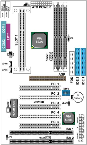
NOTE: FOR 100 / 133MHz CPU ENVIRONMENT, THE SDRAM MUST COMPLY WITH PC-100 / PC-133 SPEC.
