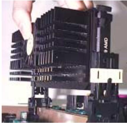
← The correct direction to insert the Heat Sink and CPU into the Heat Sink Support Frame should allow you to easily insert them.
