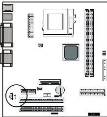
There are two audio input connectors for a CD-ROM. Plug the audio cable from a CD-ROM drive into the connector that matches the connector on the end of the cable. If there is more than one CD-ROM drive installed in the system you can connect an additional drive to the unused connector. Only one audio source at a time will play through the onboard audio subsystem.
