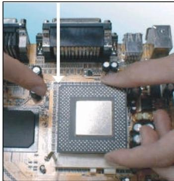
5. Lower the socket lever and press it back into place to lock the CPU in the socket.
