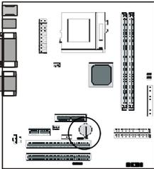
This motherboard uses a CR2032 Lithium coin battery to maintain the system configuration record created by the BIOS CMOS Setup Utility. The battery should last for several years. If the battery fails, the system will not be able to retain the system settings and will not operate properly. If this happens, do as follows:
