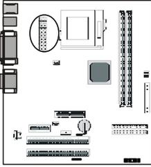
The power connector from the ATX power supply is a rectangular plastic connector with multiple wires running back to the power supply. It plugs onto the ATX power connector on the motherboard. The connector will only plug on one way, so if it won't plug on easily, turn it around and try again. Make sure the power supply is unplugged when you connect the power lead.
