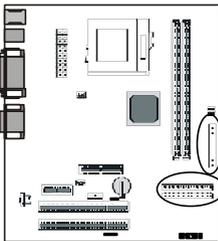
This motherboard has three connectors for disk drives, one for up to two floppy disk drives and two EIDE connectors which can connect to two IDE devices each for a total of four. The motherboard comes with two ribbon connector cables, one floppy cable and one IDE cable.
