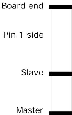
The end drive connector on the ribbon cable is for the Master IDE device and the middle connector is for the Slave device. The supplied cable supports IDE devices in all modes.
