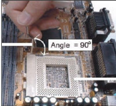
4. Insert the CPU in the socket so that the angled pin corners match the angled pin receptacle corners. The CPU will only insert in the correct orientation. Don't force it. If it doesn't go in easily, check and make sure you've got the CPU correctly oriented.
