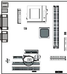
The serial port bracket plugs onto the COM2 connector on the motherboard. Mount the port bracket in an expansion slot opening that doesn't block an expansion slot and plug the ribbon cable connectors onto the connectors on the motherboard. The connectors will only plug on in one orientation so you can't get it wrong.
