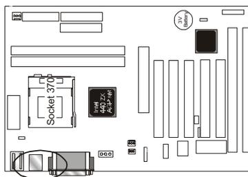
**SB LINK – For Sideband Signals Connector**
