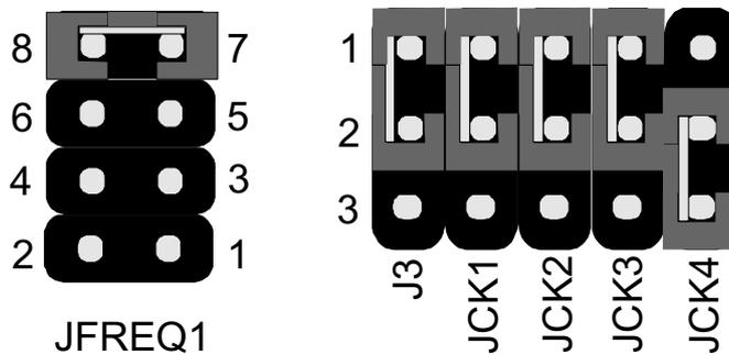
**CPU Bus Speed – 100MHz part (SDRAM Frequency is 66.6MHz)**
