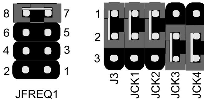
**CPU Bus Speed – 100MHz part (SDRAM Frequency is 100MHz)**
