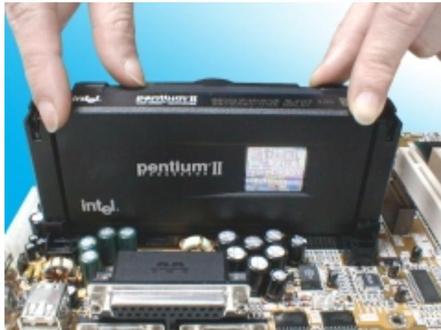
**Note:** Some Slot 1 processors with different packing maybe need the caps to let them be fixed. So if it need the caps during installing Slot 1 CPU, please follow this step: “ Fix the CPU locking caps onto the two ends of the CPU stays ”.
