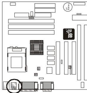
**Audio Jacks – For Line-In, Line-Out, Mic. Connectors**
