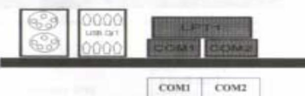
The onboard serial connectors are 9-pin D-type connector on the back panel of mainboard.
