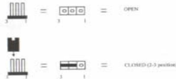
NOTE: When you open a jumper, attach the plastic jumper cap to one of the pins to you won't lose it.
