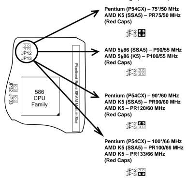
Figure 2–1–1. CPU Jumper Settings
