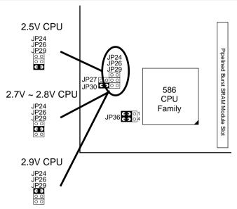
Figure 2-2-2. Dual Voltage CPU
