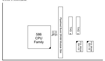
Figure 2–3–1. 256K Pipelined Burst Cache Configuration
