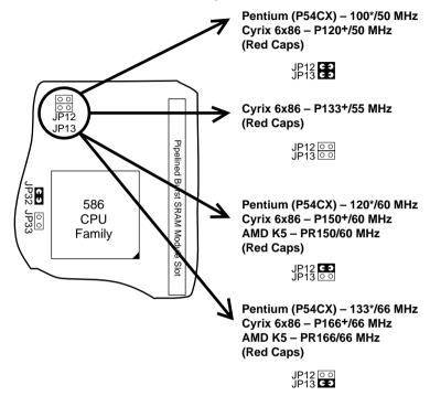
Figure 2–1–2. CPU Jumper Settings
