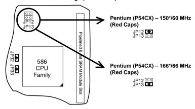
Figure 2–1–3. CPU Jumper Settings
