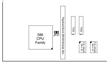
Figure 2–3–2. 512K Pipelined Burst Cache Configuration
