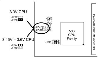
Figure 2–2–1. Single Voltage CPU
