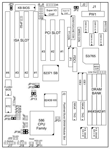
Figure 1–2. Mainboard Default Setting
