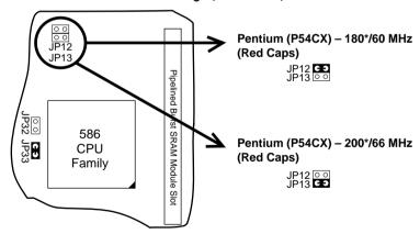
Figure 2–1–4. CPU Jumper Settings
