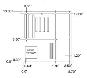
Figure 1. Advanced/AS Motherboard dimensions
