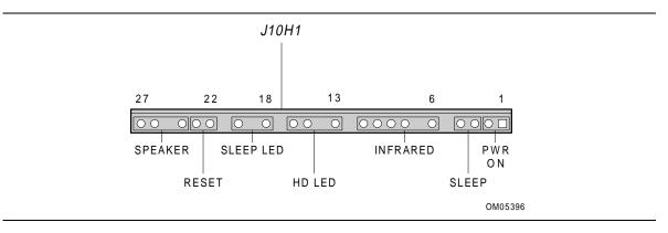
Figure 4. Front Panel I/O Connectors (J10H1)
