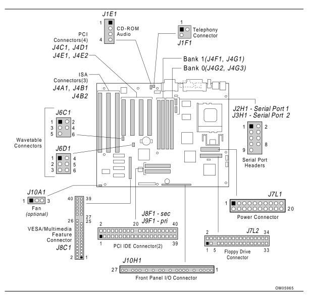
Figure 3. Motherboard Connector Locations
