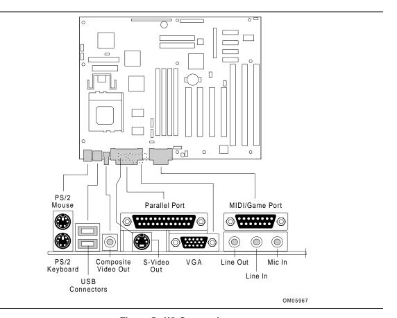
Figure 5. I/O Connections
