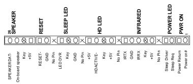
Figure 3: Front Panel I/O Connector, J27 (1 x 26 header)
