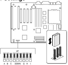
Figure B-1. Location of configuration jumpers.
