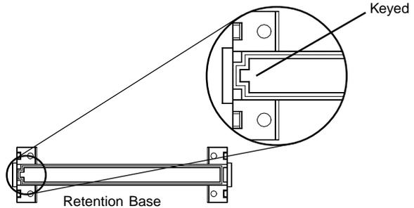
3. Using a screwdriver, tighten all four sides of the Retention Base.
