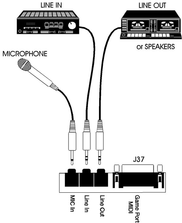
Figure 3-7: Connecting External Sound Devices
