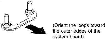
2. Place the Retention Base over the Slot 1 connector and insert it down into the Support Bridges with studs. Note the “Keyed” location of both Slot 1 and the Retention Base.
