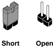
This illustration shows a 2-pin jumper. When the jumper cap is placed on both pins, the jumper is **SHORT**. If you remove the jumper cap, or place the jumper cap on just one pin, the jumper is **OPEN**.
