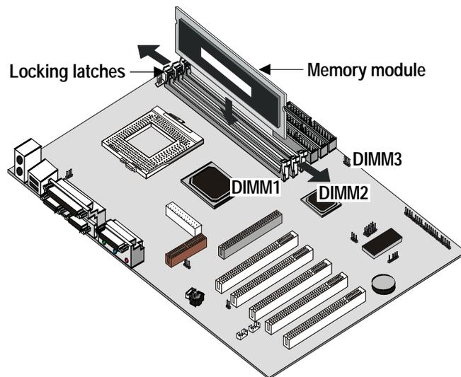
2. The DIMM slots are keyed with notches and the DIMMs are keyed with cutouts so that they can only be installed correctly. Check that the cutouts on the DIMM module edge connector match the notches in the DIMM slot.
