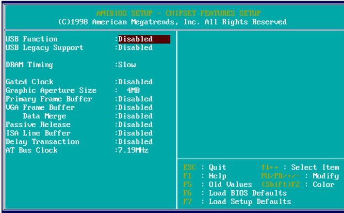
This setup page is used to specify advanced features available through the chipset. The default settings have been chosen carefully for the most operating conditions.
