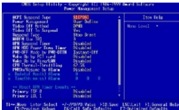
Each power-saving mode has a respective timer. The value of the timer can be assigned or reloaded and it will count down to zero. When the timer equals to zero, the system will be forced into the related suspend or power-saving mode. If any predefined signal or event is detected during the timer counting period, the timer restarts automatically.
