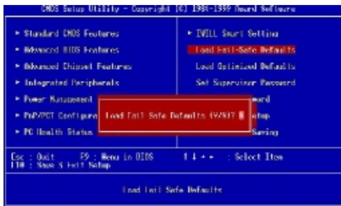
Pressing 'Y' loads the BIOS default values for the most stable, minimal-performance system operations.
