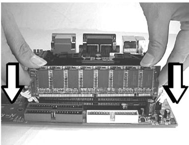
**Step 3: Press the latches into the notches of the RAM module.**
