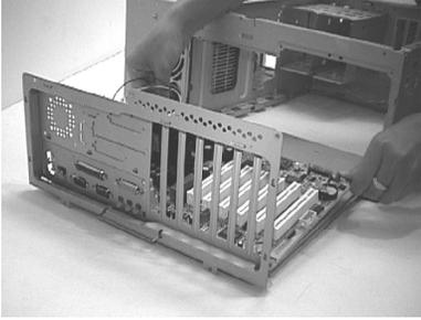
**Step 3:** Insert the expansion card into the PCI socket
