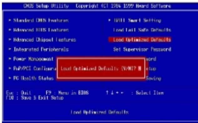
Pressing 'Y' loads the default values that are factory settings for optimal performance system operations.
