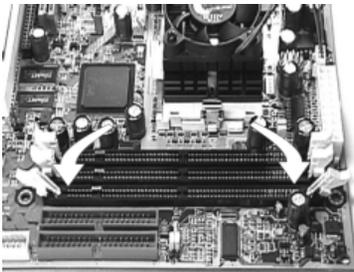
**Step 2:**Proofread the RAM module to the DIMM Socket
