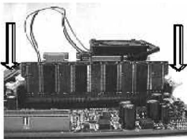
Insert the RAM module into the DIMM socket.
