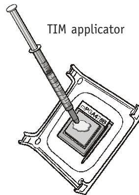
2. Do not spread the TIM around. When you place the Heatsink on top of the CPU the material will disperse evenly.
