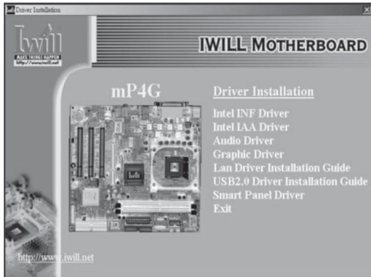
Install the first two items for the Intel Chipset, Intel INF Driver and Intel IAA Driver, in sequence by clicking on them and following the install program instructions.
