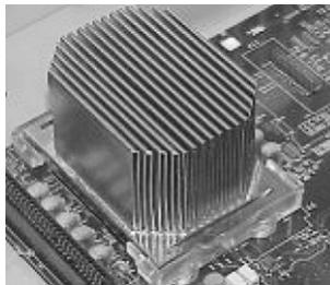
Don't spread the TIM out with the applicator tip. Wiggle the Heatsink a little after you position it to disperse the Thermal Interface Material.
