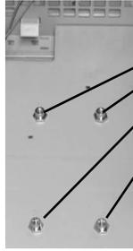
There are four Retention Mechanism mounting standoffs for each CPU socket on an EEB 3.0 housing's motherboard mounting plate.
