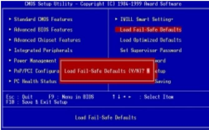
Pressing ‘Y’ loads the BIOS default values for the most stable, minimal-performance system operations.
