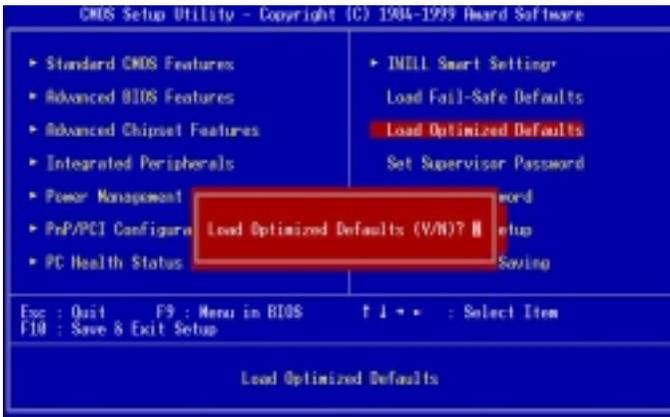
Pressing ‘Y’ loads the default values that are factory settings for optimal performance system operations.
