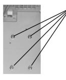
There are four Retention Mechanism mounting standoffs for each CPU socket on an EEB 3.0 housing's motherboard mounting plate.
