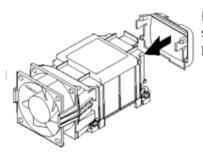
Press the end cap into the shroud so that it snaps into place securely
