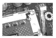
Match the Pin 1 positions on the socket and the processor
