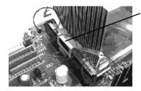
position the clip so that the large tab is on the outside and fits over the mechanism extension there
