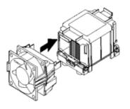
Press the fan mount into the shroud so that it snaps into place securely
