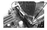
Hold the clip down in the middle while you press the each end of the clip onto the Retention Mechanism
