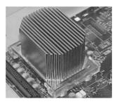
Don't spread the TIM out with the applicator tip. Wiggle the Heatsink a little after you position it to disperse the Thermal Inteface Material.
