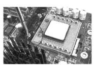
Insert & tighten the mounting screws so that they screw into the CPU backplate
