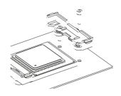
Position the mechanism facing in towards the CPU socket.
