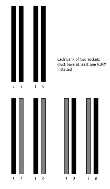
Installing RIMM or CRIMM modules is simple. The modules insert in the sockets and are held in place by the socket retaining arms. The edge connectors on the modules are of different widths and there are key notches in the center of each module. These ensure that you can not insert a module incorrectly.
