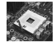
Raise the socket lever to the vertical position
