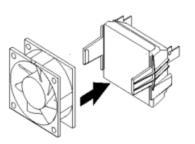
Orient the fan so that it blows toward the Heatsink 2. Insert the fan mounting frame tabs into the holes on the forward side of the PWT Shroud. The plastic tabs should snap securely into place.
