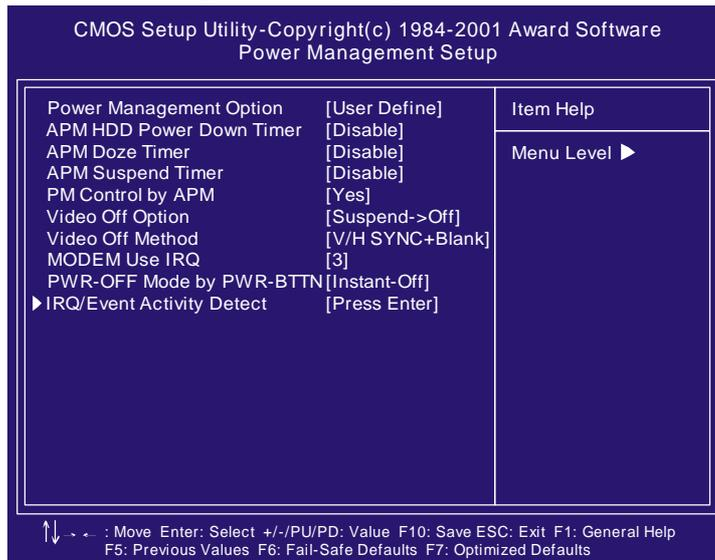
Each power-saving mode has a respective timer. The value of the timer can be assigned or reloaded and it will count down to zero. When the timer equals to zero, the system will be forced into the related suspend or power-saving mode. If any signal or event is detected during the timer counting period, the timer restarts automatically.
