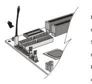
Detects system temperature. NO NEED to contact this thermostat to any device. Leave it on the motherboard.
