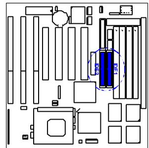
You may configure two hard disks to be both Masters using one ribbon cable to the primary IDE connector and another ribbon cable on the secondary IDE connector. You may install one operating system on an IDE drive and another on a SCSI drive and select the boot disk through the BIOS Setup.
