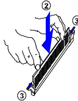
2. Install the DIMM straight down into the DIMM slot with both hands.
