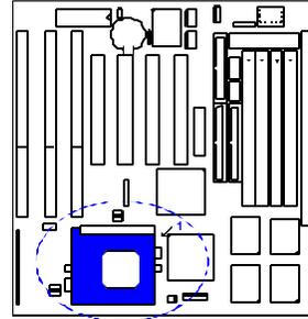
**NOTE :** Without a fan circulating air on the CPU and heat sinks, the CPU and/or heat sinks can overheat and cause damage to both the CPU and the mainboard.
