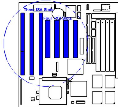
**NOTE :** Before installing an expansion card, make sure to unplug the power supply when adding or removing expansion cards or other system components. Failure to do so may cause severe damage to both the mainboard and expansion cards.
