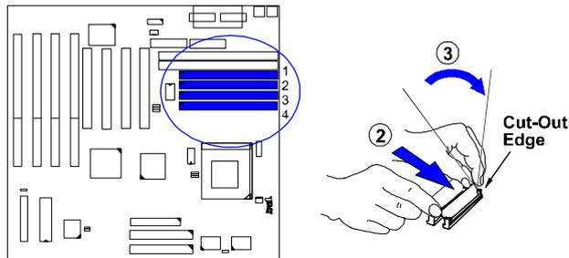
**NOTE** : SIMMs in each bank must be of the same type; and the BIOS automatically configures the memory size.
