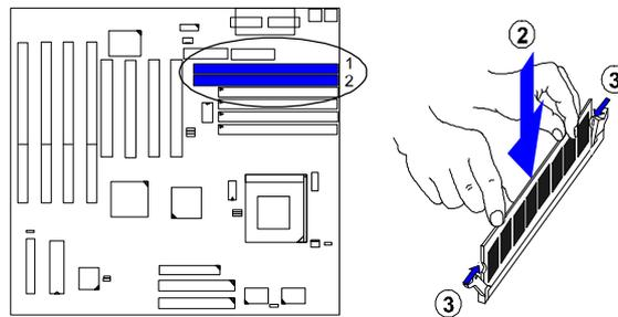
2. Install the DIMM straight down into the DIMM slot with both hands.
