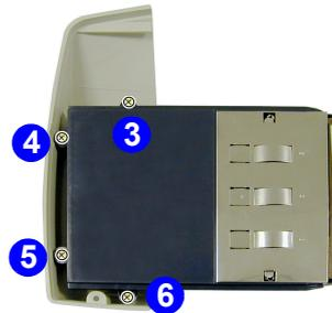
5. Remove screws ① - ⑥ which hold the hard disk to the case, and slide the hard disk out.
