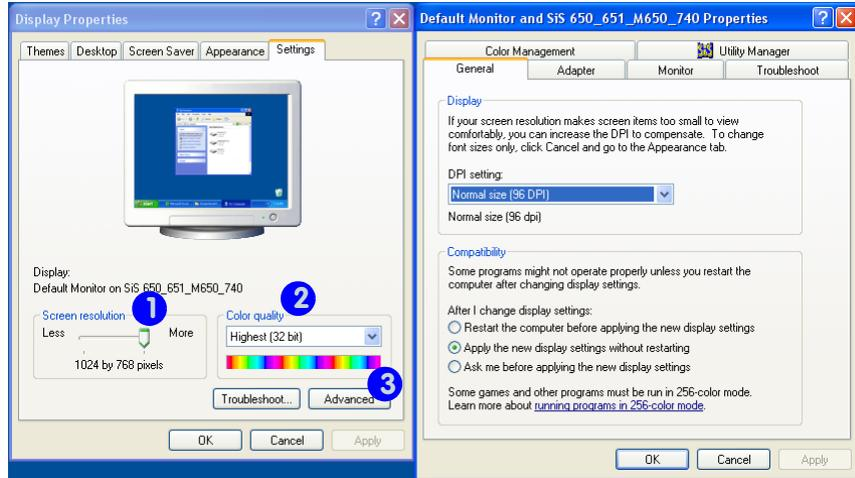
When the **Display Properties** control panel is open, click the **Advanced** **3** (button) to bring up the options tabs. Clicking through these tabs allows you to make any video adjustments you require.
