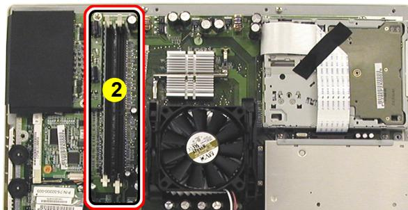
5. The memory sockets will now be visible at point **2** on the mainboard.
