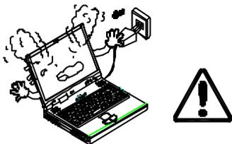
*Unplug the power cord when attaching peripheral devices.*
