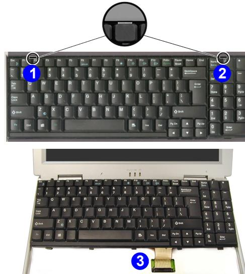
3. Lift the keyboard up and out, being careful not to twist the keyboard ribbon cable **3**.
