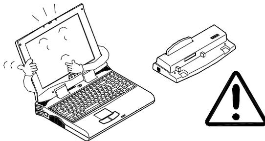
*Unplug the power cord before attaching any peripheral devices.*
