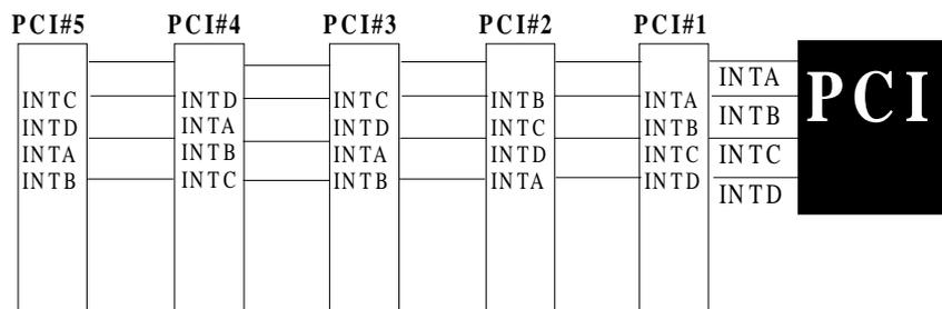
**Figure 3-7: The Combination of PCI INT#lines**
