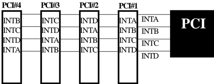
**Figure 7: The Combination of PCI INT# lines**
