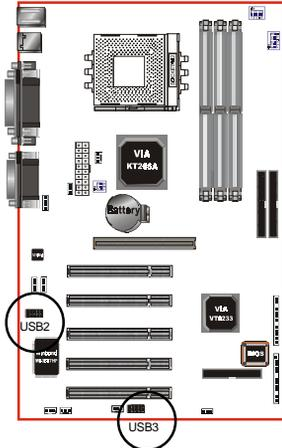
**USB2/3:** USB port header pins for share with four USB ports.
