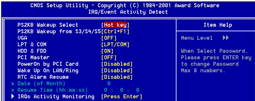
**PS2KB Wakeup Select :** This item allows you to select Hot Key or Password to wake-up the system by PS2 Keyboard. When select Password, please press ENTER key to change password max 8 numbers.
