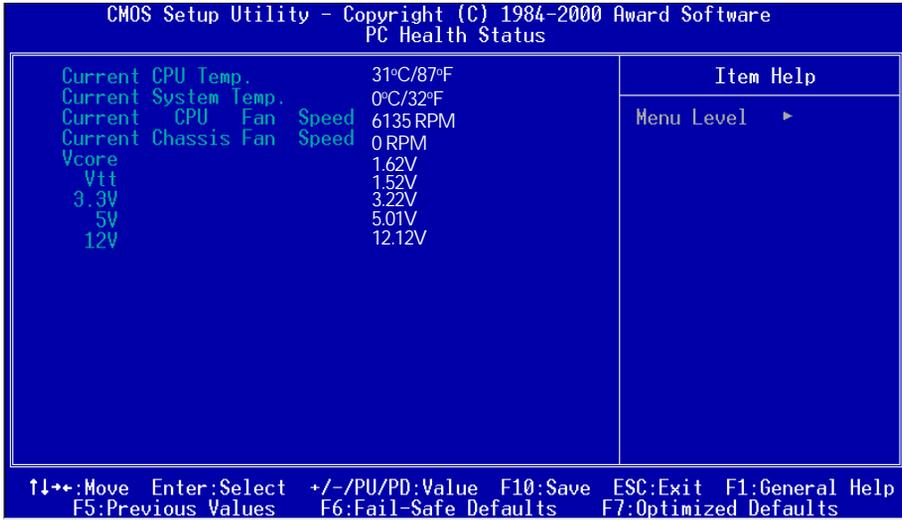
**Current CPU Temperature:** This is the current temperature of the CPU.
