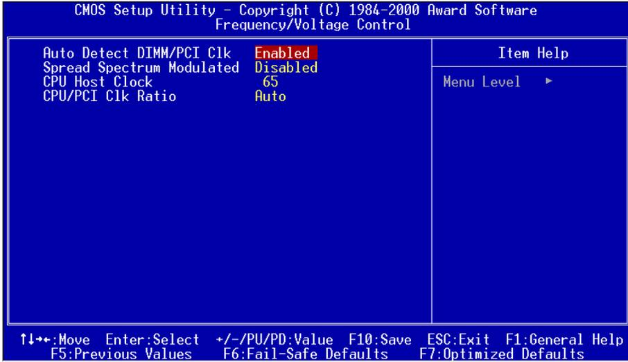
**Auto Detect DIMM/PCI Clk:** When enabled the motherboard will automatically disable the clock source for a DIMM socket which does not have a module in it. Same applies for PCI slots. The default is Enabled.
