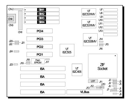
Locations of Jumpers and Connectors on the G586VPA System Board
