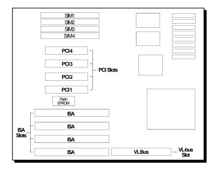
The system board supports three Master slots. The function of PCI3 and PCI4 is both Master and Slave. PCI1, PCI2 and VL-Bus slots share the function of the third Master slot. If you insert a Bus Master card into one of these slots (PCI1, PCI2 or VL-Bus) then the other two slots can support Slave function only.
