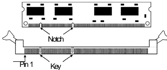
1. Pull the "\_\_\_" which are at the ends of the socket aside.
