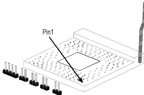
3. Position the CPU above the ZIF socket. Make sure pin 1 of the CPU is aligned with pin 1 of the socket. Lower the chip until the pins are inserted properly in their corresponding holes. Remember that very little force is needed to install the CPU. If the CPU is not easily inserted, verify whether or not pin 1 of the CPU is aligned with pin 1 of the socket. Applying too much pressure can damage the CPU or the socket.
