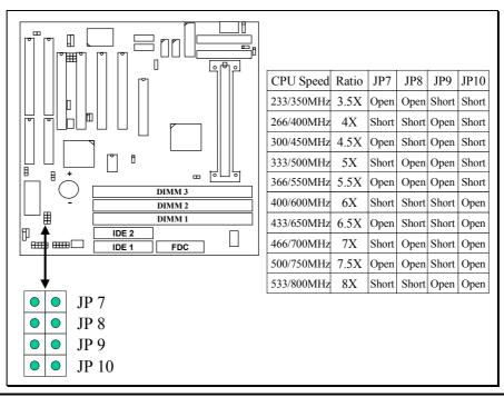
Basically, there are two parameters which will decide the CPU speed - the Front Side Bus (FSB) speed and CPU clock ratio. When you have installed the processor onto the mainboard, the system BIOS will detect the CPU type and decide the FSB speed automatically (please refer to **section 4-6** – "CPU Host Clock (CPU/PCI)"). As for the clock ratio, it is selected by the jumper setting on JP7, JP8 and JP9 as shown above.
