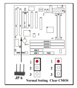
Note: Improper BIOS setting may cause PC system hang-up, In case that it happened, use JP4 to clear the CMOS information and get the PC system back to normal. Improper connection may cause permanent damage to the mainboard. Please refer to the following steps to clear the CMOS
