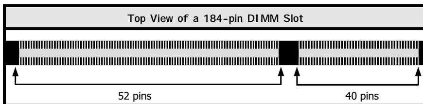
**Important:** The DIMM's can only be fitted into the slots in one orientation. Make sure that the DIMM's are in the correct orientation and the pins are correctly aligned before you insert them.
