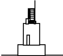
The retaining clips should fit over the edge and hold the SIMM in place.
