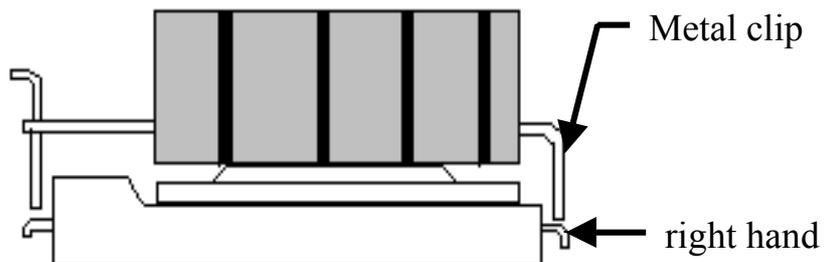
3. Hook the right hand side clip to the CPU socket first.
