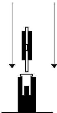
Insert the DIMM module into the socket as shown in the left picture.
