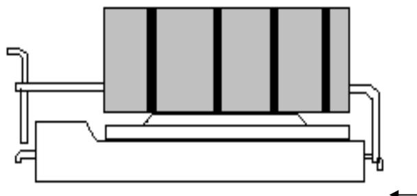
4. Push down the opposite side of the metal clip firmly and carefully to lock the cooler in place.
